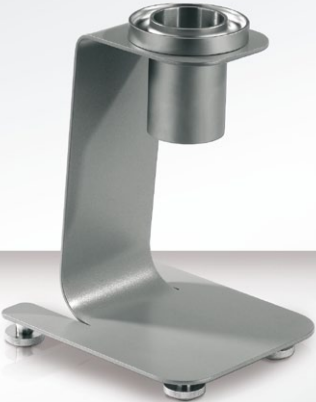
Flow Cup Viscometers with Tripod support
